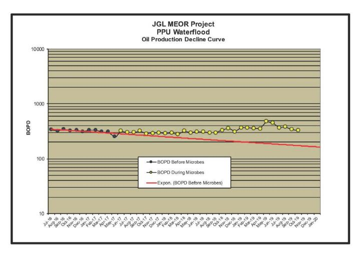
The chart above highlights the projected decline curve (red line) before the use of microbes and the actual production realized from JGL's microbial process (yellow dots).
