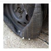
The WG Wrap and Roll Spike design works on all vehicle's types from ordinary SUV vehicles to HGV's and heavy plant type vehicles, unlike hollow type or solid type spikes the this has a fluted design that makes a large and deep puncture in the target vehicle tyres and ensures 3 points of controlled deflation per spike.
