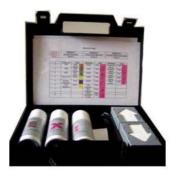
A unique, aerosol-based field test kit for the detection and identification of group-A explosives (TNT, TNB, etc.), group-B explosives (Semtex, RDX, C-4, etc.) and compounds containing inorganic nitrates that are used in improvised explosives (e.g. ANFO).
