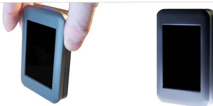
The WG POC Mobile Phone Detector will start to detect RF activity as soon as it is turned on, depending on the threshold setting that the unit is set at, it may start vibrating and displaying activity with the LED's.
