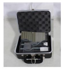
The WG ASTM F792-OE Step Wedge Test Object Case is used to calibrate and evaluate performance levels of X-ray screening systems for objective evaluation to score technical capabilities of the system per the new F792-17e1 standard. To meet the need for testing sophisticated X-ray systems, the new WG ASTM F792-OE test object is manufactured to strictly comply with the FAA, TSA, Transport Canada, and DHS requirements.
