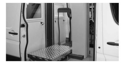
The X-ray protection shutter cuts off the X-ray radiation from the generator in case of deviations from the system mechanisms and electronic devices operation parameters and conditions set by the manufacturer as well as in case of malfunctions.
