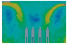
Down draughts due to oppositefacing outlets, which reduce efficiency of ventilation.
