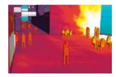
Heat intensity in case of solar radiation behind glazed surfaces, which demands cooling technology.
