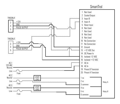
4-20 mA TRICON/E must be powered by 24 VDC. The SmartTrol is able to produce 24 VDC by "stacking" two independent 12 VDC power supplies. Configure the SmartTrol to provide +24 VDC by tying the +12 VDC (PIN 15). This jumper causes +24 VDC to appear across PIN 16 referenced to ground (PIN 12).
