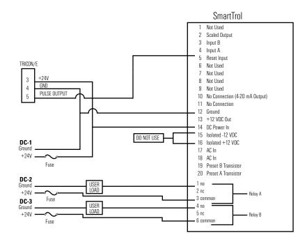
The SmartTrol may be powered by an external DC power supply. The supply must provide 12-27 VDC and at least 250 mA of current. The positive side (+DC) of the supply should be connected to terminal 14 and the negative (or ground) side to terminal 12. Units Powered by DC voltage do not have an isolated voltage on terminals 15 and 16.
