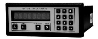
The SmartTrol is a remote instrument designed for flow rate monitoring, totalizing, and batching. It has an 8-digit, 0.55-in bright alphanumeric display. The two inputs (A and B) will accept up to 1,000 pulses per second (pps) of digital count. The two inputs are combined into a single count that can be used to provide a two-stage relay output for valve control.
