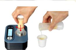
► Add 200 µL *ONE* Diluent into a new strip test vial, add 100 µL of filtered extract into the same vial, cover and mix well by shaking 3 times.
