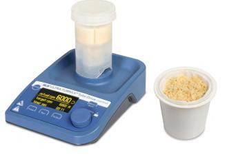
Strips must be stored at at 2-30 °C (36-86 °F) Store AQUA Premix at room temperature Peanuts: Limit of Detection 2 ppb, Range: 0-100 ppb Peanut Paste: Limit of Detection 1.5 ppb, Range: 0-75 ppb
