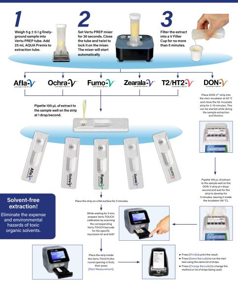
Calibration only needs to be scanned once per lot. Instrument stores calibration.
