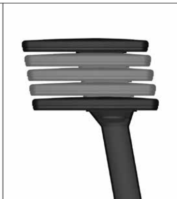
Height Adjustment • 12 Positions • 4 3/8" Range of Motion
