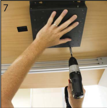
Mount the Switcher Box shelf in place using #6 x 5/8" screws (qty 4).
