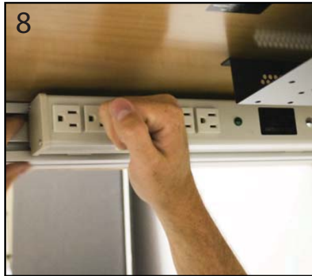
With the supplied plastic tabs snapped into place on underside of Surge Protector, align with grooves in support rail and gently push into place (qty 1).
