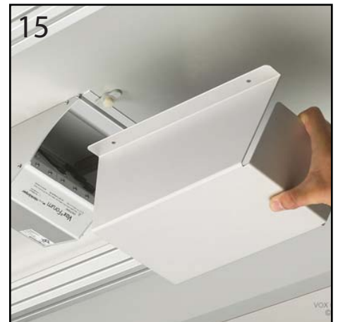
Manage all "Show Me" cables with Wire Management trays. To install, position closely to Forum and screw in place with #6 x 5/8" wood screws (qty4).
