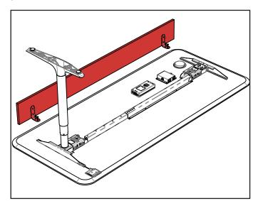
If your desk includes a partial modesty panel, attached modesty brackets to panel with #8 x 5/8" pan head wood screws. Attach assembly to top with 1/4"-20 x 7/8" joiner bolts.
