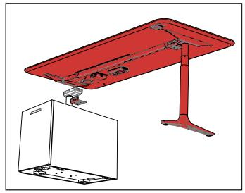
Carefully align pedestal mounted column with leg cradle in frame. Lower in place and fix with leg clamp and lock described previously.
