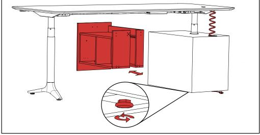
Cables route from desk top through case by feeding curly cord through pedestal and out the pedestal bottom. To do this remove drawer by squeezing lock triggers under front lip of drawer. This disengages slide locks. Case and legs can be leveled by turning installed glides to desired height.
