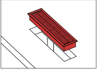
If your desk includes a rectangular grommet, insert unit into hole in top and secure with screw included with grommet packaging.
