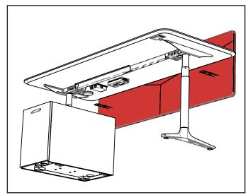
If your desk includes a divider, align brackets pre-installed in divider with inserts in underside of top. Fix with 1/4"-20 x 7/8" joiner bolts. Dividers can be positioned tight to desk or with cable gap.
