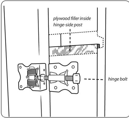
**ezTIP:** Before installing hinges, determine which way you want gate to swing. Hinges and latch striker will be mounted on the same side of gate posts.
