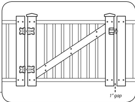
Hang gate so that there is a 1" opening on latch side of the gate. This can be accomplished by tightening or loosening the nuts on the T-Rod on the hinges. BOTH nuts on the T-Rod MUST be tightened or loosed together. Attach latch to the post to receive the latch striker.
