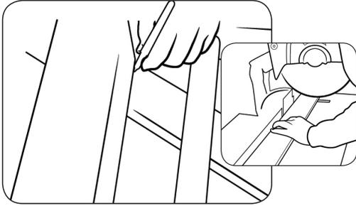
Mark brace to fit snug when placed diagonally between gate posts.
