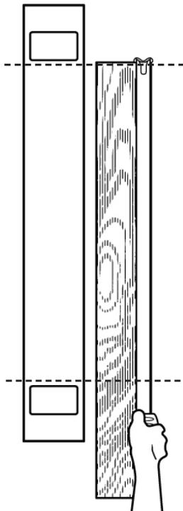
Gate Post: Measure distance between routed holes on side of railing gate post and mark on plywood insert  $\frac{1}{2}$ " shorter than the distance between the routed holes.
