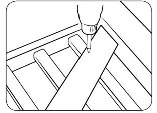
Insert 2 screws and screw caps through brace into center picket and pickets closest to posts. Be sure to not over tighten!
