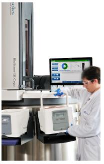
cellular structures from degradation. BioStore™ III Cryo is an automated cryogenic storage system that maintains samples at -190°C. BioStore III integrates with inventory management systems, tracks the temperature of all samples, protects innocent samples from warming during retrieval, restricts sample access to predefined users and provides complete inventory tracking and audit trail.
