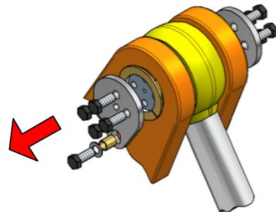
1.1.3/ Assemble the tool as shown. The jaws should be fixed to the flange on the conical sleeve. Use a spanner and rotate the sliding screw clockwise. The conical sleeve will be pulled out.
