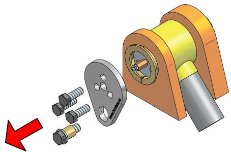
3.1.3/ Assemble the tool as shown. The jaws should be fixed to the flange on the conical sleeve. Use a spanner and rotate the sliding screw clockwise. The conical sleeve will be pulled out.
