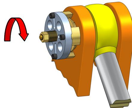
1.1.4/ When the conical sleeves are removed on both sides, the pin can be pulled out.
