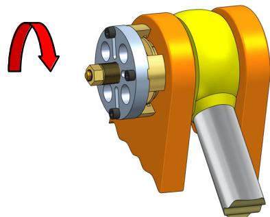
3.1.4/ When the conical sleeves are removed, the pin can be pulled out.
