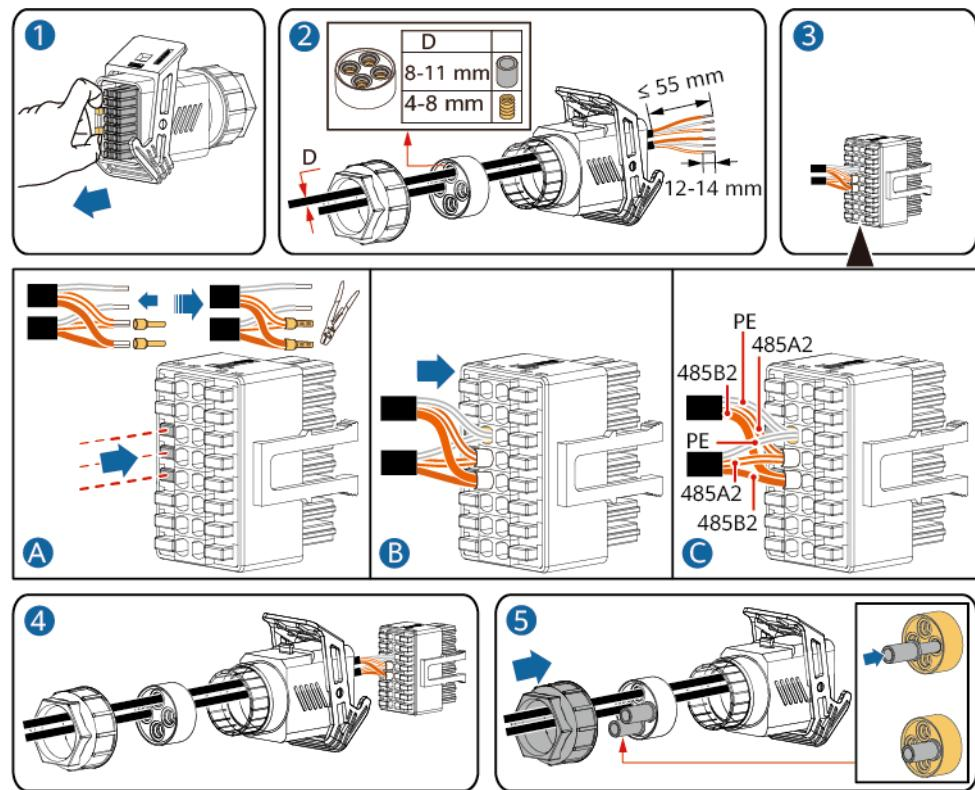
**Step 2** Connect the signal cable connector to the COM port.
