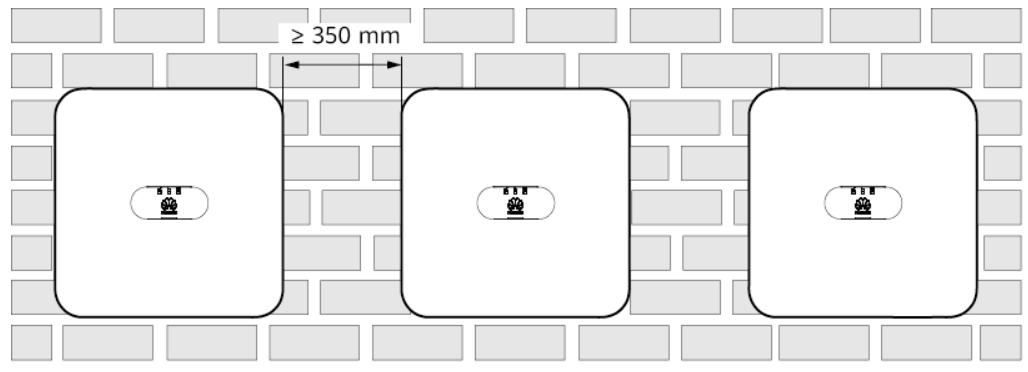
**Figure 4-4** Staggered installation (recommended)
