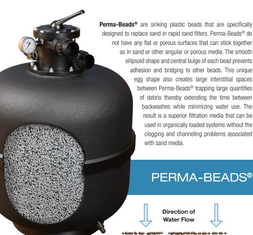
Perma-Beads® are sinking plastic beads that are specifically designed to replace sand in rapid sand filters. Perma-Beads® do not have any flat or porous surfaces that can stick together as in sand or other angular or porous media. The smooth ellipsoid shape and central bulge of each bead prevents
