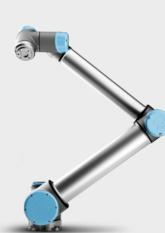
$<sup>^{\</sup>star}$  The robot can work in a temperature range of 0-50 °C. At high continuous joint speed, ambient temperature is reduced.
