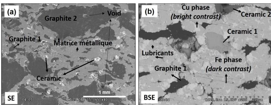
Microstructure of simplified semi-metallic brake-pad material. a) Secondary electrons image at low resolution, b) Backscattered-electrons at higher resolution
