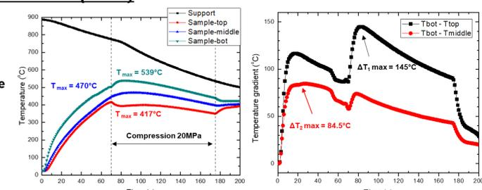
Schema of experimental approaches with sample which has dimension of 20x20x20mm and temperature gradient measured by inserted thermocouples, 3 different signals correspond to different position on sample (top, middle, bottom)
