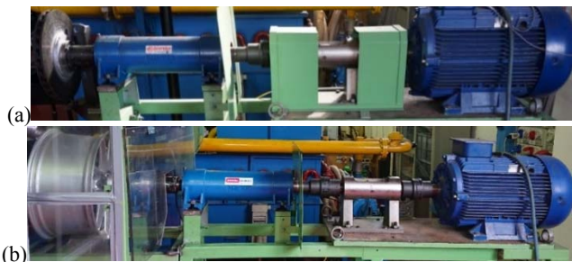
Figure 6 (a) the existing test bench, (b) the developed test bench.
