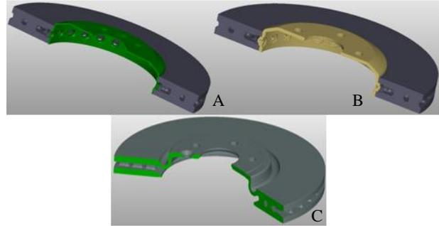
Figure 3 Comparison of the brake disc geometries: A plug-in with steel hub; B plug-in with aluminium hub; C conventional cast iron design
