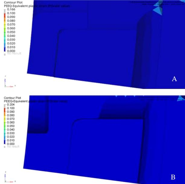
Figure 9 Detailed view on the locking pin at the time point of highest thermal loading: A assembly with steel hub; B assembly with aluminium hub
