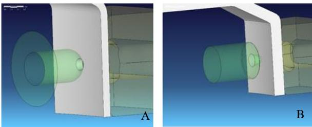
Figure 11 Model setup for the forming simulation: A steel hub; B aluminium hub
