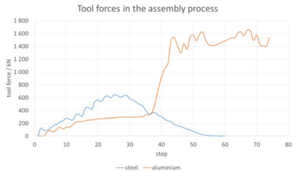
Figure 13 Tool force diagram for the forming simulation of the steel and aluminium hub
