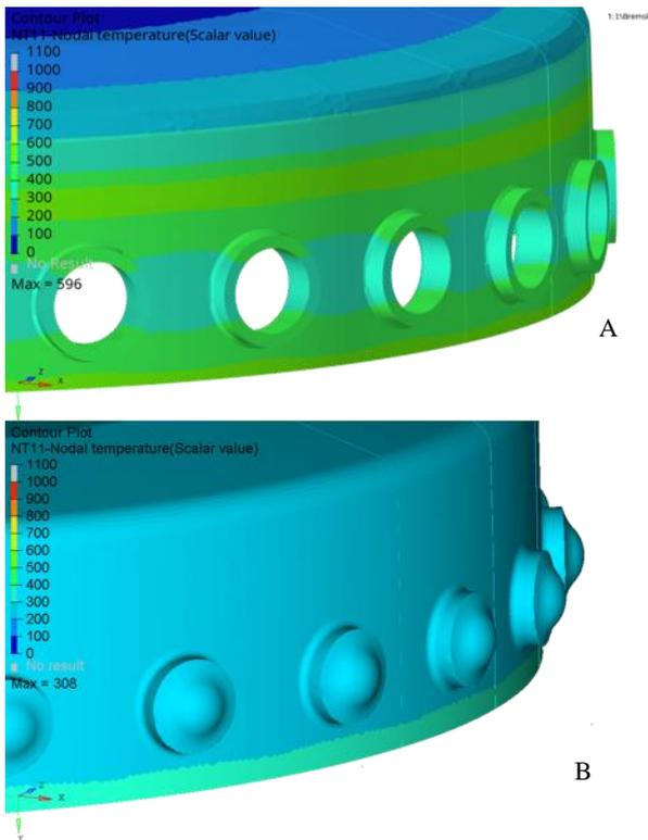
Figure 8 Temperature distribution on the hub in the time point of the highest thermal loading: A steel hub; B aluminium hub
