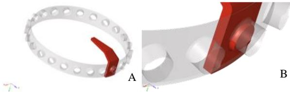
Figure 5 Example model to determine the misuse braking torque of a plug-in assembly: A general overview; B detailed view on a locking pin
