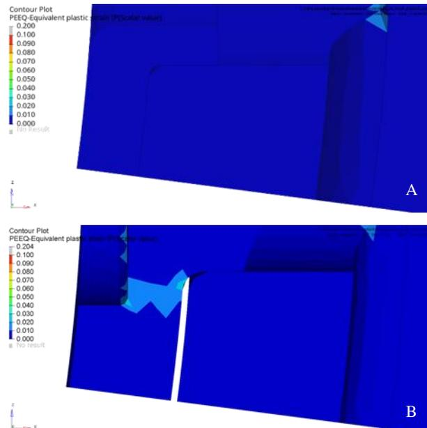
Figure 10 Detailed view on the locking pin at the end of the calculated loading cycle: A assembly with steel hub; B assembly with aluminium hub
