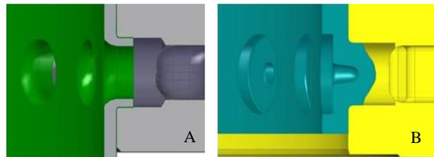
Figure 4 Locking pins in the plug-in brake discs: A steel hub; B aluminium hub
