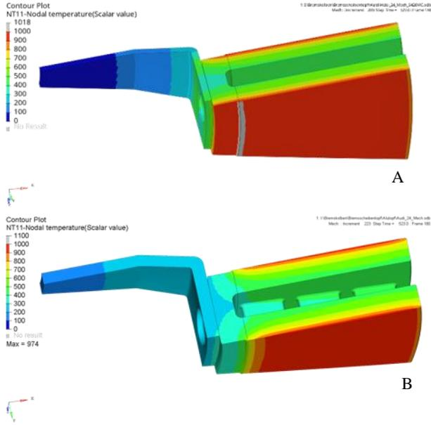
Figure 7 Temperature distribution in the time point of the highest thermal loading: A assembly with steel hub; B assembly with aluminium hub
