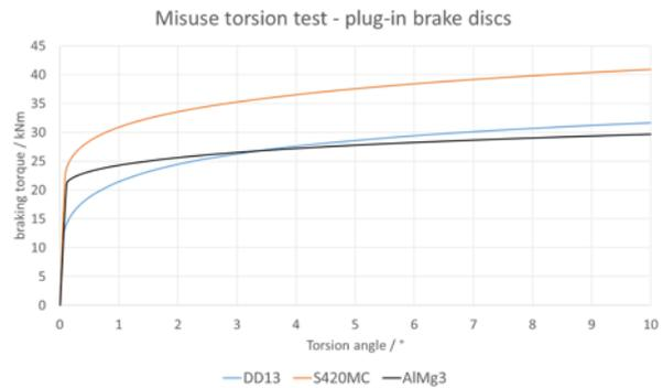
Figure 6 Torque – angle diagram for the misuse test of plug-in brake discs
