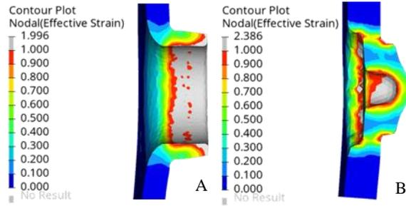
Figure 12 Plastic deformation resulting from the finite element forming simulation: A steel hub; B aluminium hub
