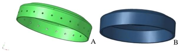
Figure 2 Comparison of the plug-in brake disc hubs: A steel hub with 2.5 mm material thickness; B aluminium hub with 5.0 mm material thickness
