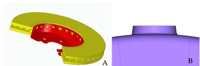
Figure 1 Geometry of the plug-in brake disc with the steel hub: A section view of an example assembly; B detailed look at a single locking pin at the hub
