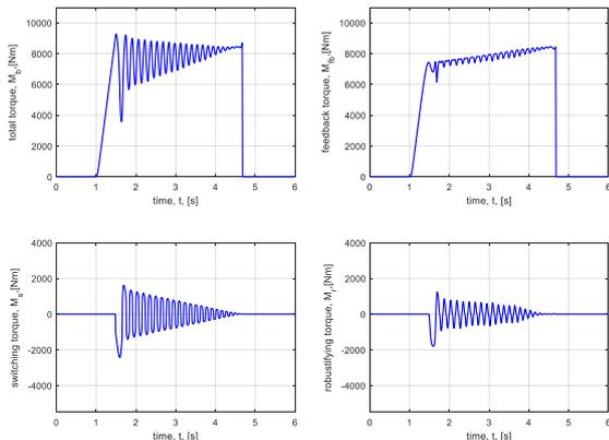
Figure 5. Total, feedback, switching and robust torques from controller (d)-scenario 1
