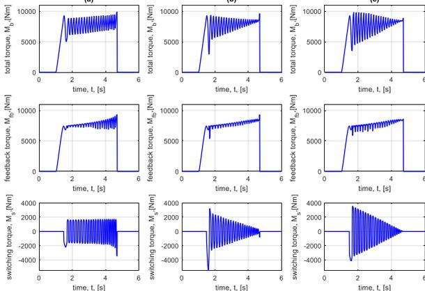
Figure 4. Total brake torques and its components controllers (a) to (c), scenario 1
