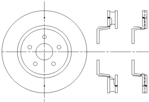
Figure 2 Embedded Thermocouple Installation
