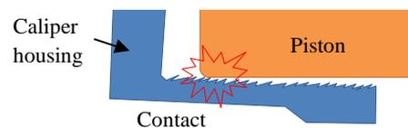
Figure 16: Piston touching BUE deposits on the caliper housing piston bore
