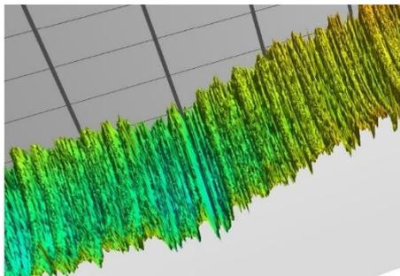
Figure 19: Area ①: 3D surface analysis of Part © - without BUE deposits - Enlarged
