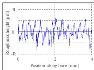
Figure 8: Surface profile of Part ② (without visible machining lines)
