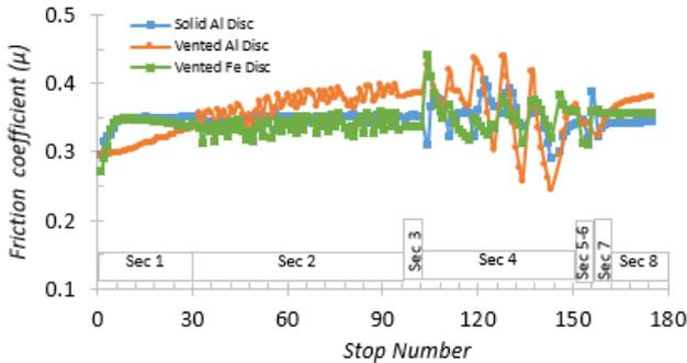
Figure 3 Average friction coefficient values of coated discs compared to cast iron disc at 100°C IBT
