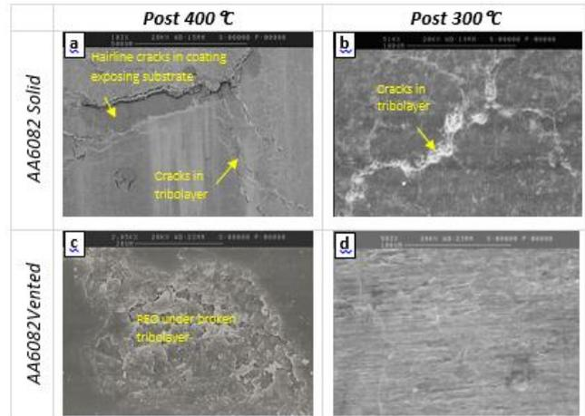
Figure 7 SEM micrographs of disc surfaces after the AK master test of 1800 stops.
