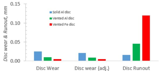
Figure 5 Disc wear and Runout measurements of various discs tested up to 400°C.
