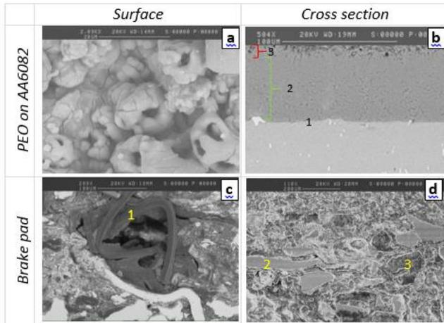
Figure 2 SEM images of the PEO coating on Al disc: a) as coated free surface, b) cross section showing ‘3’ top porous layer, ‘2’ main technological layer and ‘1’ interfacial layer; and c) brake pad free surface, d) brake pad cross section. 1- Fe; 2 – Cu Zn; 3 – Al Si
