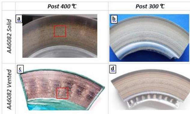
Figure 6 Photographs showing surfaces of coated discs after 400°C and 300°C brake test
