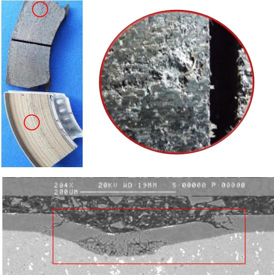
Figure 9 Micrographs vented Al disc after brake test at 300°C showing: a) gouging on the coated Al disc surface caused by hard steel wire on the brake pad; b) brake pad showing above hard steel wire used as a reinforcing material; c) BSE cross sectional image of the gouge showing the substrate plastically deformed together with the PEO coating and still maintaining strong coating adhesion.
