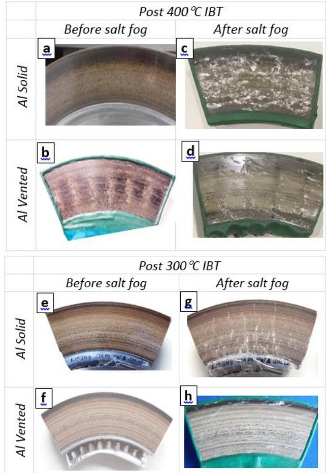
Figure 10 Photographs showing surfaces of the brake discs before corrosion testing and after exposure to 68 hrs of salt fog corrosion. Vented disc shows only very little superficial corrosion
