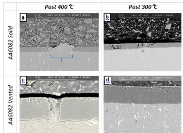
Figure 8 SEM micrographs of Al disc cross sections after the AK master test of 1800 stops.
