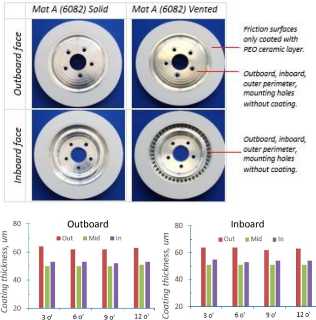
Figure 1 PEO coated discs prior to dynamometer testing (top) and coating thickness distributions across the rubbing outboard and inboard surfaces (bottom).
