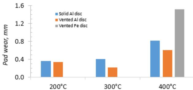
Figure 4 Pad wear values against various Al and iron discs
