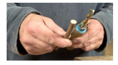
Use and hand drill to drill a hole three quarters of the way through the centre of the base disc. Push down and twist.
