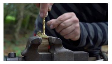
You can also use an electric drill to do this to. Clamp the tree top firmly on its side to your bench, then drill the hole. Make sure you line up the drill to avoid miss-hitting the clamp or bench.
