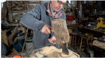
Using the mallet apply a soft tap to make a groove. Then hit harder to split the disc in half. Take each half and again split each one in half. This will give you four quarters, so four tree tops.
