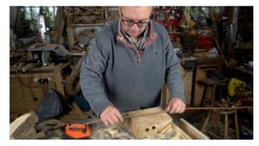
Select a section of approx 10cm and place the craft knife on top of the stick on the chopping block. Push down with the craft knife and twist the other end of the stick at the same time. This will make a clean cut. You can choose a thinner or thicker trunk as you like.
