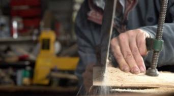
Attach the piece of firewood to the edge of your table or bench with a G-clamp or secure it in a vice. Now saw off your 15-20mm tree shape slice.
