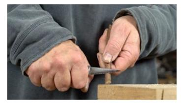
If you happen to whittle off too much and the trunk is now too small, cut off a small piece of the tapered end of the stick using the knife or a saw. Again start to whittle to find the snug fit we're looking for.
