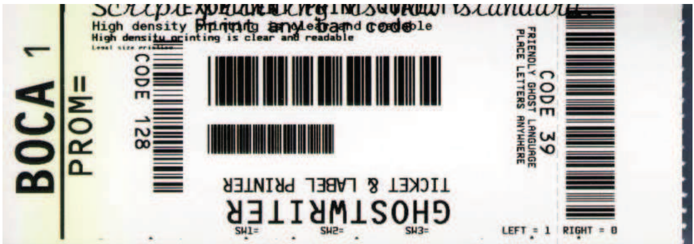
Above sample FGL ticket was printed on a 2" x 5.5" (concert) ticket using a RADJW-2" 200dpi FGL printer.
