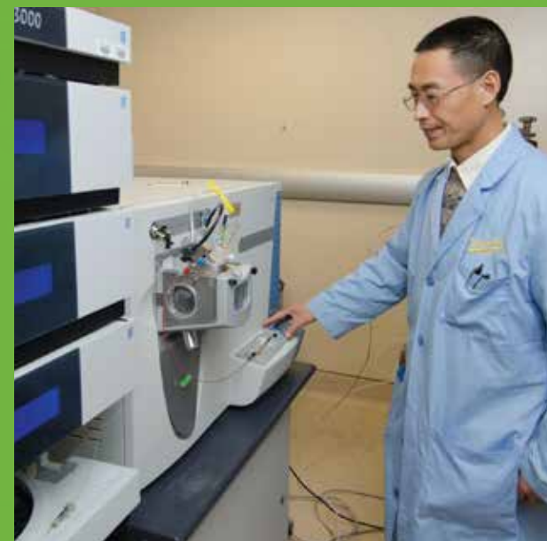
Qiang Zhang, Ph.D. Ultra-high performance liquid chromatography (UPLC) LTQ Orbitrap XL Mass Spectrometer by Thermo. See New Major Instrumentation story on page 10.
