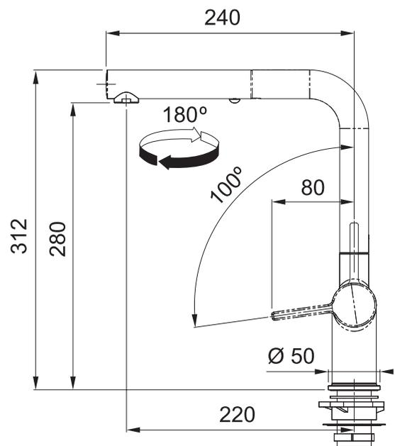
**PLEASE NOTE:** Large and heavy taps should ideally be mounted directly through the solid benchtop or fully supported from underneath. For all other swivel taps, we recommend the use of the Franke Tap Support Arm to provide additional support. Please ensure all Franke tapware is installed at a pressure of no greater than 500 kPa in accordance with AS/NZS3500 and insist that your plumber flushes all of the water supply lines before installing tapware. Failure to do so may void warranty.
