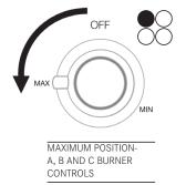
2. Press and hold the control knob down firmly for a full 5 seconds to ensure the flame failure device engages. If the flame goes out after you release the knob then the flame failure device did not engage – simply press down the knob firmly again turn to max position and keep pressing for a full 5 seconds.
