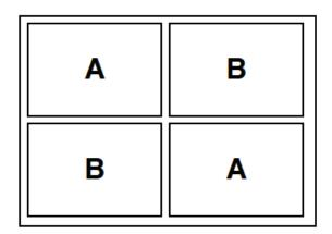
If the selected heating levels for both zones exceed the maximum available amount of power, the power management function is automatically reducing the power from one of these zones. The display of this zone is first blinking; the level is then automatically reduced to the highest suitable position.
