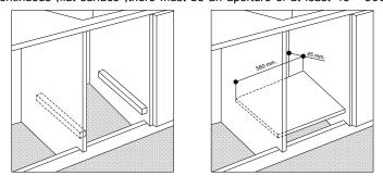
The panels of the adjacent cabinets must be made of heat-resistant material .In particular ,cabinets with a veneer exterior must be assembled
