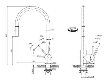
**PLEASE NOTE:** Large and heavy taps should ideally be mounted directly through the solid benchtop or fully supported from underneath. For all other swivel taps, we recommend the use of the Franke Tap Support Arm to provide additional support. Please ensure all Franke tapware is installed at a pressure of no greater than 500 kPa in accordance with AS/NZS3500 and insist that your plumber flushes all of the water supply lines before installing tapware. Failure to do so may void warranty.
