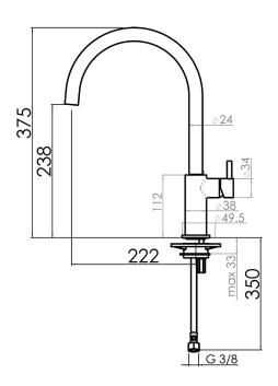
**PLEASE NOTE:** Large and heavy taps should ideally be mounted directly through the solid benchtop or fully supported from underneath. For all other swivel taps, we recommend the use of the Franke Tap Support Arm to provide additional support. Please ensure all Franke tapware is installed at a pressure of no greater than 500 kPa in accordance with AS/NZS3500 and insist that your plumber flushes all of the water supply lines before installing tapware. Failure to do so may void warranty.
