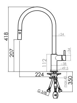
**PLEASE NOTE:** Large and heavy taps should ideally be mounted directly through the solid benchtop or fully supported from underneath. For all other swivel taps, we recommend the use of the Franke Tap Support Arm to provide additional support. Please ensure all Franke tapware is installed at a pressure of no greater than 500 kPa in accordance with AS/NZS3500 and insist that your plumber flushes all of the water supply lines before installing tapware. Failure to do so may void warranty.
