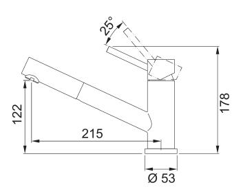
**PLEASE NOTE:** Large and heavy taps should ideally be mounted directly through the solid benchtop or fully supported from underneath. For all other swivel taps, we recommend the use of the Franke Tap Support Arm to provide additional support. Please ensure all Franke tapware is installed at a pressure of no greater than 500 kPa in accordance with AS/NZS3500 and insist that your plumber flushes all of the water supply lines before installing tapware. Failure to do so may void warranty.
