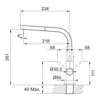
**PLEASE NOTE:** Large and heavy taps should ideally be mounted directly through the solid benchtop or fully supported from underneath. For all other swivel taps, we recommend the use of the Franke Tap Support Arm to provide additional support. Please ensure all Franke tapware is installed at a pressure of no greater than 500 kPa in accordance with AS/NZS3500 and insist that your plumber flushes all of the water supply lines before installing tapware. Failure to do so may void warranty.
