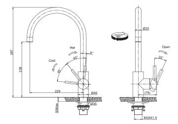
**PLEASE NOTE:** Large and heavy taps should ideally be mounted directly through the solid benchtop or fully supported from underneath. For all other swivel taps, we recommend the use of the Franke Tap Support Arm to provide additional support. Please ensure all Franke tapware is installed at a pressure of no greater than 500 kPa in accordance with AS/NZS3500 and insist that your plumber flushes all of the water supply lines before installing tapware. Failure to do so may void warranty.
