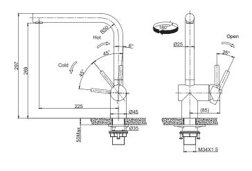
**PLEASE NOTE:** Large and heavy taps should ideally be mounted directly through the solid benchtop or fully supported from underneath. For all other swivel taps, we recommend the use of the Franke Tap Support Arm to provide additional support. Please ensure all Franke tapware is installed at a pressure of no greater than 500 kPa in accordance with AS/NZS3500 and insist that your plumber flushes all of the water supply lines before installing tapware. Failure to do so may void warranty.
