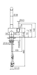
**PLEASE NOTE:** Large and heavy taps should ideally be mounted directly through the solid benchtop or fully supported from underneath. For all other swivel taps, we recommend the use of the Franke Tap Support Arm to provide additional support. Please ensure all Franke tapware is installed at a pressure of no greater than 500 kPa in accordance with AS/NZS3500 and insist that your plumber flushes all of the water supply lines before installing tapware. Failure to do so may void warranty.
