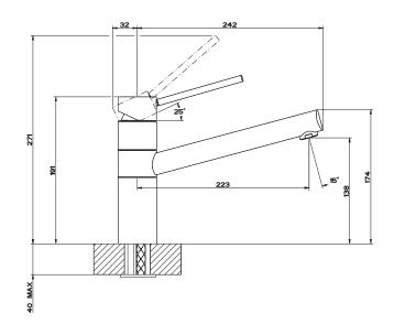
**PLEASE NOTE:** Large and heavy taps should ideally be mounted directly through the solid benchtop or fully supported from underneath. For all other swivel taps, we recommend the use of the Franke Tap Support Arm to provide additional support. Please ensure all Franke tapware is installed at a pressure of no greater than 500 kPa in accordance with AS/NZS3500 and insist that your plumber flushes all of the water supply lines before installing tapware. Failure to do so may void warranty.
