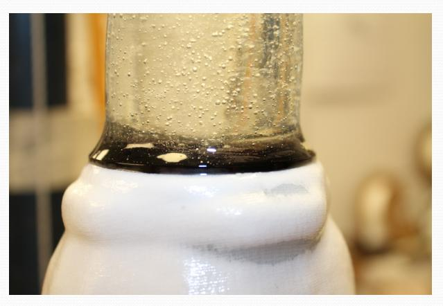
The resin should start to be sucked into the hole in the center first, not along the outside edge. Note wetting out starting
