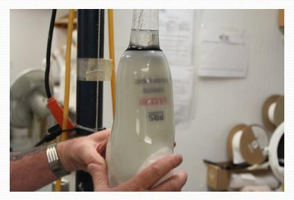
At this point, I have applied no string to this model. I've used my hands only to bring the resin slowly down through the fabric. I stop bringing the resin down at my proximal trim lines for the finished socket.
