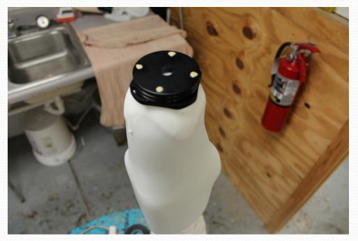
Enlarge the center hole in the distal attachment to about ½". Make a hole if there isn't one already. This hole will allow the resin to pull through the end and saturate all of the material completely
