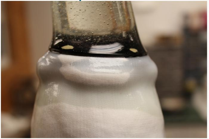
Give the resin a chance to be pulled through the distal attachment and completely saturate the fabric. DO NOT Squeeze the PVA yet.
