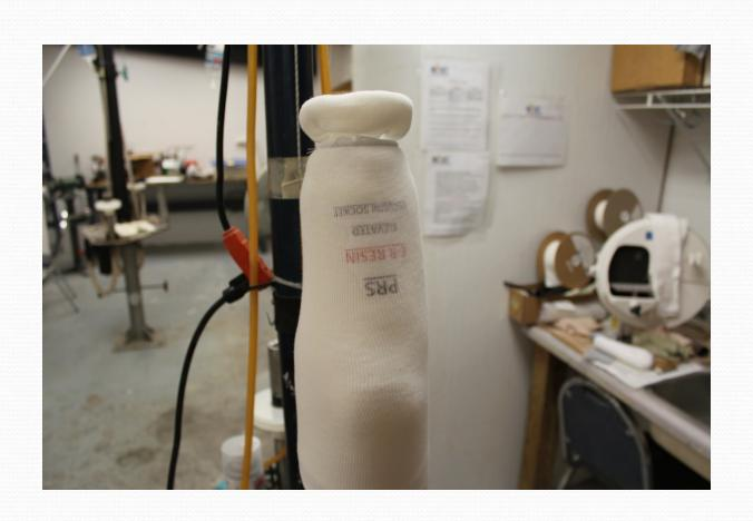
Pull your final PVA bag over the layup with the shiny side in. Make sure the PVA seals around the outer ridge of the Distal attachment and that NO fabric is over the distal end. You can apply a very thin layer of Vaseline or wax to aid in removing the excess resin from the distal end. Very Thin. Fill the bolt holes with plumbers putty too. Don't Forget!!!
