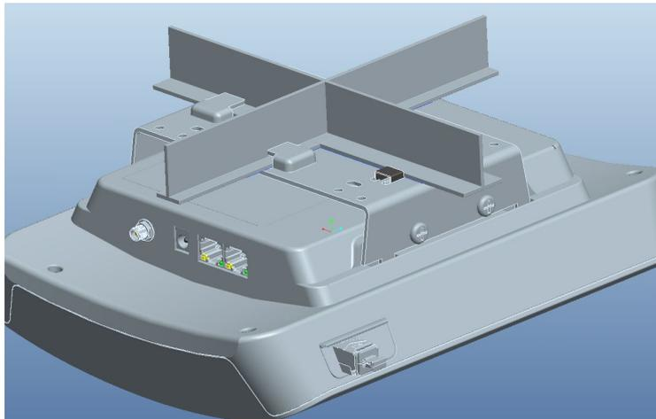
For hard-surface mounting, attach the bracket to the hard surface using the included screws with the bracket arms for the AP extending vertically upward.
