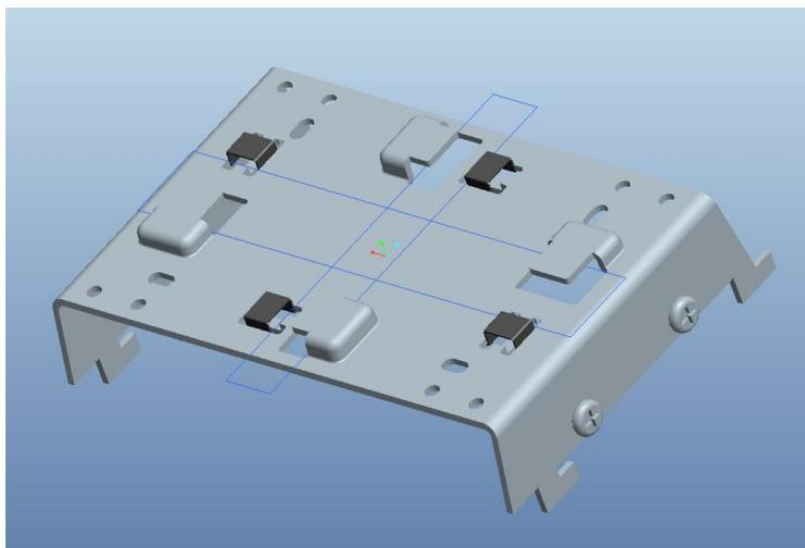
For drop-ceiling mounting, position the rear clips on the mounting bracket to the ceiling grid and twist counter-clockwise until the springs lock into place. Two sets of rear clips on the mounting bracket support both 24mm and 15mm T-grid rails.
