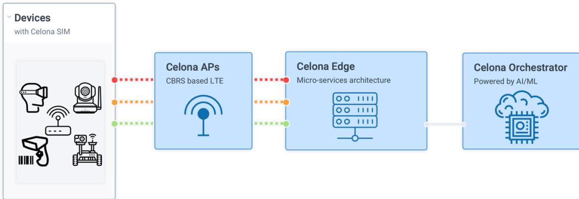
The system consists of the essential functions detailed in Figure 1: System Architecture. The Celona Orchestrator performs AP authentication, validates the AP's serial number, determines the network the AP needs to connect to and finally directs the Celona Indoor AP to the serving Celona Edge.
