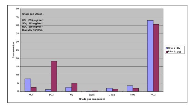
Ill 6: Comparison of gas cleaning systems "wet" and conditioned dry" (2005)
