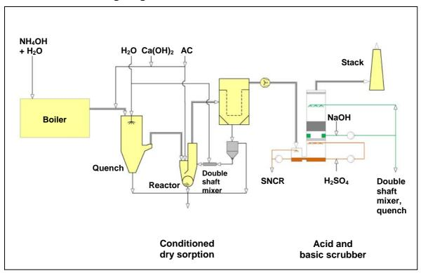
III. 7: TwinSorp process: Variant I: Combination of conditioned dry sorption – acid scrubbing
