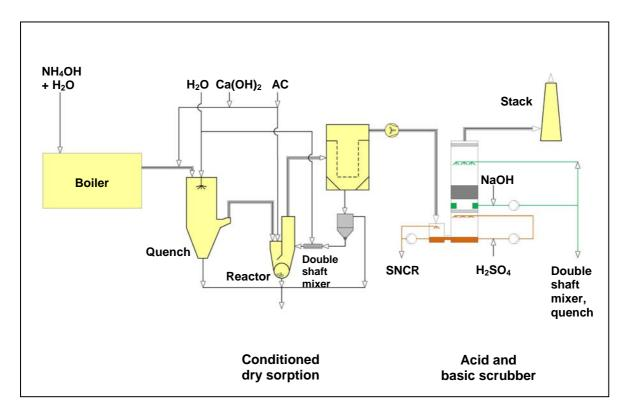
III. 8: TwinSorp process: Variant II: Combination conditioned dry sorption – acid and basic scrubbing
