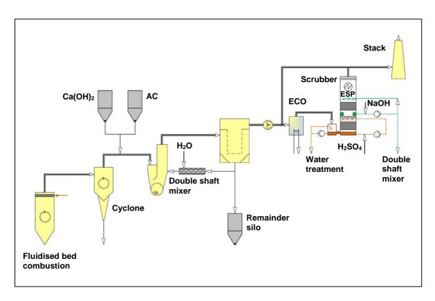
III. 11: Process concept for gas cleaning system at HVC Alkmaar
