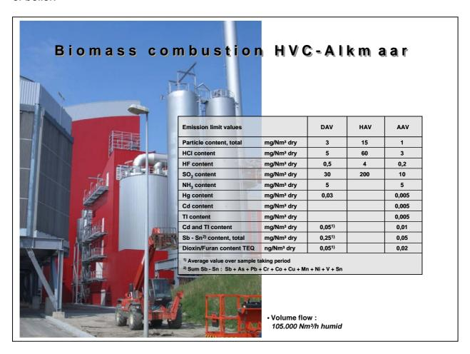
III. 10: Gas cleaning downstream biomass combustion at HVC in Alkmaar
