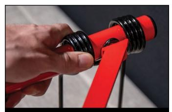
Slide the brace down to the bar and line up the drill hole of the brace to the tine and drill hole on the bar.
