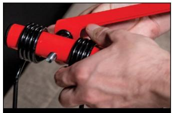
**Do not tighten the nuts on the brace at this time.**
