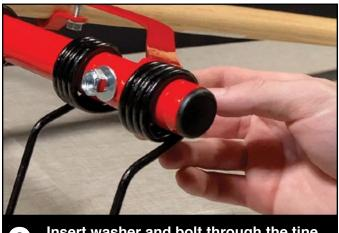
Insert washer and bolt through the tine, bar, and brace.
