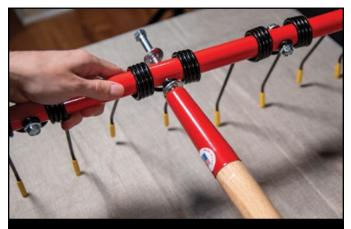
Insert lag screw through middle tine and into the handle.
