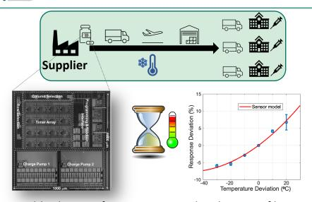
Enables battery-free, continuous data logging of historical conditions such as temperature, vibration, or light
