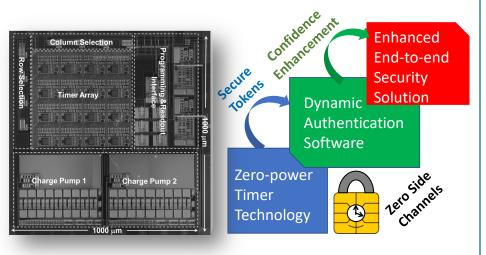
Ultra-secure root-of-trust for resource constrained internetof-things (IoTs) like sensors and wearables
