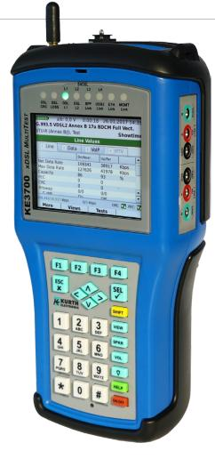
The KE3700 xDSL *MultiTest* is the next evolution in the KE-*MultiTest* series. In addition to all established features, it also has brand-new functions and functionalities like Wi-Fi testing, Bluetooth-supported data transfer and touchscreen functionality as well as a optimized rubber keyboard and shortcut keys.
